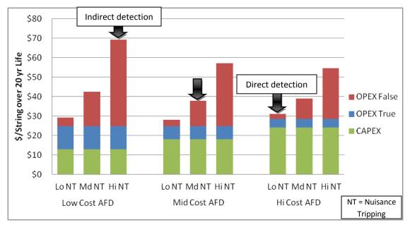
The black arrows indicate the likely outcomes with each type of detector. For instance, as discussed in the performance section (section 4.2), the lower cost AFD architectures will tend to have more nuisance tripping than the higher cost ones. Therefore, the high nuisance tripping case is most likely for the low cost version and vice versa for the high cost one, as shown by the black arrows.
