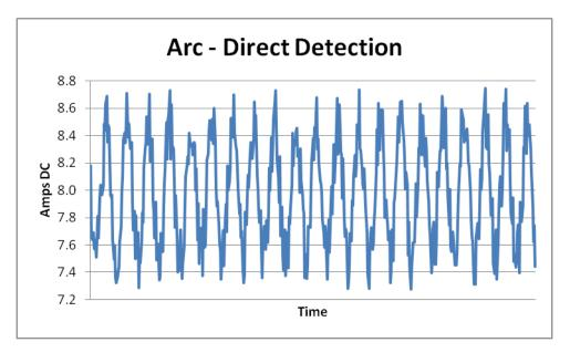
Alternatively, when an arc exists in a string with indirect detection, the signal observed by the AFD in a 16 string combiner box would appear as below. The arc signal is 1/17 of the strength of the signal in the direct detection architecture. This indirect detection signal is only slightly different from the background noise and makes distinguishing the arc from background noise using this signal very difficult and greatly increases the risk of nuisance tripping.
